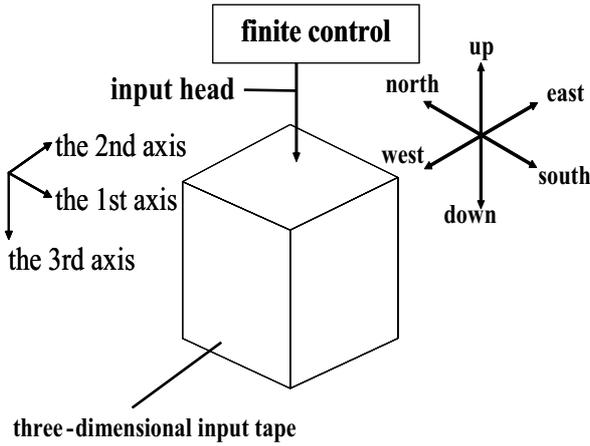
Fig. 2: Three-dimensional finite automaton.
